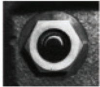
B. PARTIALLY FULL Replace at the next maintenance interval
